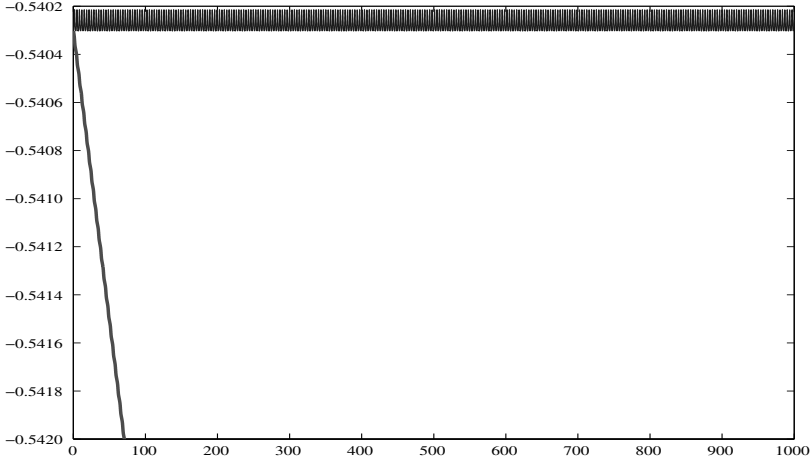
Figure 5.6 The Hamiltonian energy \frac{1}{2}y_{n,2}^2 - \cos y_{n,1} , as rendered by the implicit midpoint rule (the narrow band extending across the top of the figure) and the Nystrom method (the steeply sloping line).
